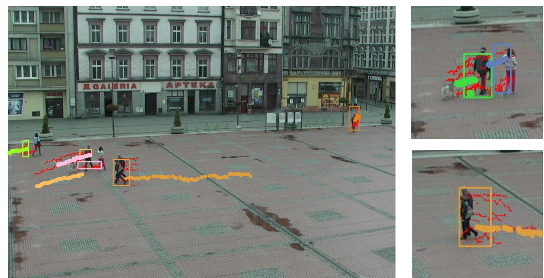
Fig 3. Path clustering procedure applied on a video sequence from Bytom Market Square. Red lines indicate paths, colour bold lines join cluster centres over consecutive frames, rectangles are cluster contours in the current frame. Too low distances between silhouettes prevents them from being separated by the clustering algorithm (right-bottom figure).
